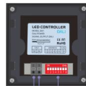
Power and Signal Combined Socket      Dip Switch
