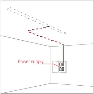
1 | Make the electrical connection to the power supply and then run the wires to the location of the light fixture.
