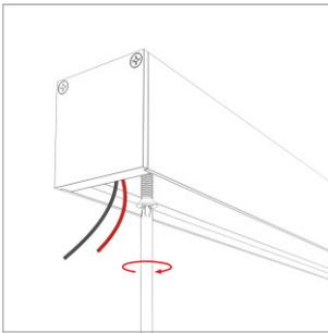
4 | Run the wires through the hole, then secure the fixture into the surface.
