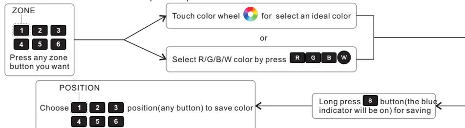
For example, press zone button 1, then touch color wheel for orange color, then press S button (the blue indicator will be on), then choose position button 3. That's to say, we save orange color from zone 1 into position 3.
